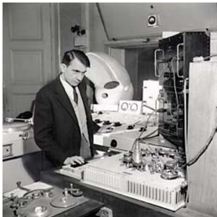
Pierre Schaeffer in 1952 playing the phonogène à clavier , a tape recorder with its speed altered by playing any of twelve keys on a keyboard.
